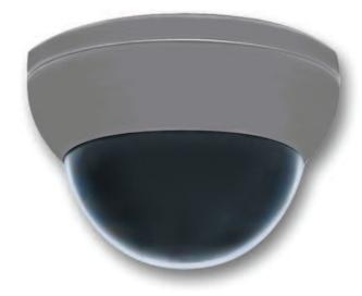
Our color vandal resistant dome camera operates on a 24V AC power supply, which allows line lock and adjustable phase. It offers HAD technology and a 3-9mm auto iris varifocal lens. Additional features include a low smear level, which prevents glare in dark conditions, pre-set auto exposure and turbo AGC (automatic gain control). The heavy duty housing is built to withstand the blows from a 10 pound sledge hammer. Also available in white housing (CVC-7245EXTP/W)
